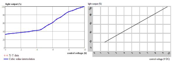
Figure 6 Light output variation related to control voltage:
