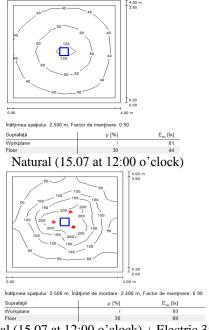
Natural (15.07 at 12:00 o'clock) + Electric 35% **Figure 7** Lighting levels 15.07 TDGS/Hybrid System
