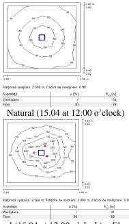
Natural (15.04 at 12:00 o'clock) + Electric 40% Figure 6 Lighting levels 15.04 TDGS/Hybrid System
