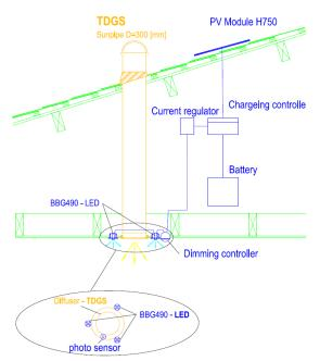
Figure 1 Composition of the proposed hybrid system
