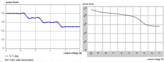
**Figure 8** Power factor variation related to control voltage: a – interpolation for the 150 W SON-T lamp; b – provided by the manufacturer
