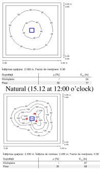
Natural (15.12 at 12:00 o'clock) + Electric 70% **Figure 5** Lighting levels 15.12 TDGS/Hybrid System
