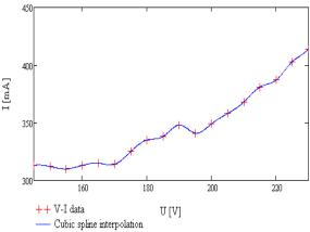
**Figure 3** V-I characteristic of the studied lighting assembly
