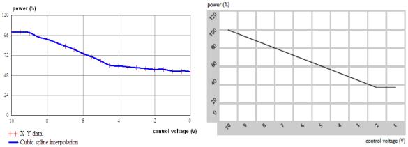
Figure 7 Active power variation related to control voltage:
