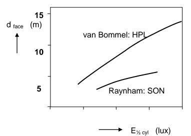
Figure 3 Identification distance d, under residential area lighting circumstances in dependence of semicylindrical illuminance  $E^{1/2}$ cyl, with white high pressure mercury light HPL and with yellowish high pressure sodium light. Raynham [8].
