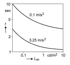
**Figure 1** Time (t) required to response to a change in angle of a lead car as function od the average road surface luminance Lav. Fisher and Hall [3].
