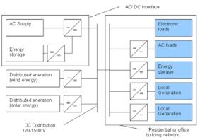
Figure 1 LVDC network with distributed generation units [1]
