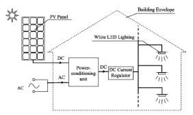
Figure 5 DC Lighting System using LED's [5]
