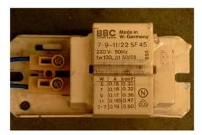
**Figure 1** One and the same ballast is designed for four different single lamps and three possible tandem configurations (for reasons of space only one listed here). Current ratings are slightly lower for higher lamp power ratings!
