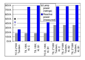
**Figure 6** Power factor as the ratio of active power (grey benches) plotted against reactive power (blue benches) for 18 W lamps and different ballasts, single and tandem modes (for comparison, 2\*9 W tandem mode also included)
