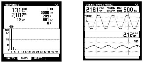
Figure 3 Harmonic current spectrum – LPN150 Figure 4 Voltage and current waveforms – LPN150
