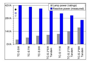
**Figure 5** Power factor as the ratio of active power (grey benches) plotted against reactive power (blue benches) for different TC-S lamps from 5 W to 11 W with the same ballast, single and tandem modes
