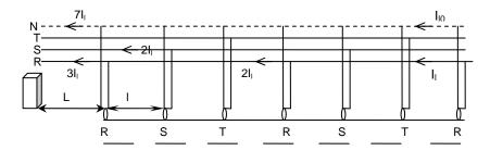
Figure 5 Public lighting network – electrical connection and currents flow
