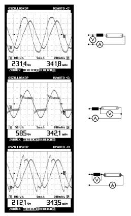
Figure 4 Voltages across a fluorescent lamp and a magnetic ballast
