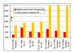
**Figure 9** 18 W fluorescent lamps in single and tandem mode (for comparison, 2\*9 W tandem mode from Figure 8 also included)
