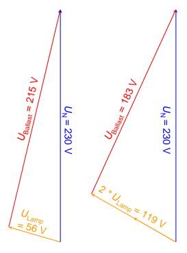
**Figure 3** Simplified vector diagram for single and tandem mode operation of a 5 W TC-S lamp – it seems that 2\*56 V=119 V in this case but this is because current is slightly lower in tandem mode, which makes lamp voltage greater!
