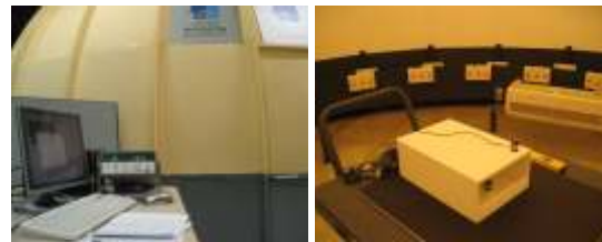
(a) measurement system (b) scale model Figure 7 Measurement of illuminance
