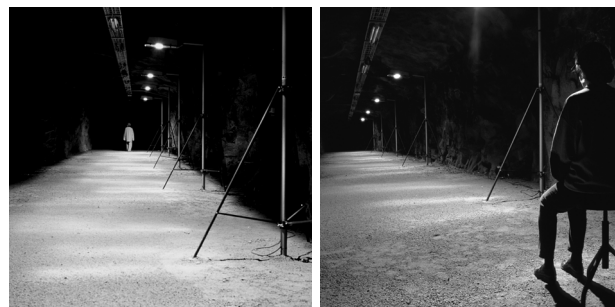
Figure 4. Pedestrian visibility measurements in underground road lighting installations. The subject indicated with a response button when she/he could detect the walking pedestrian 40...50 m apart.
